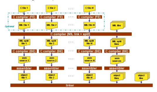
To read more about how MIL linking influences the build process of your application, see Section 9.2, *MIL Linking*.
