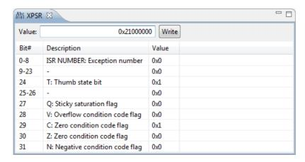
In this view you can set the individual values in the register, either by selecting a value from a drop-down box or by simply entering a value depending on the chosen field. To update the register with the new values, click the **Write** button.
