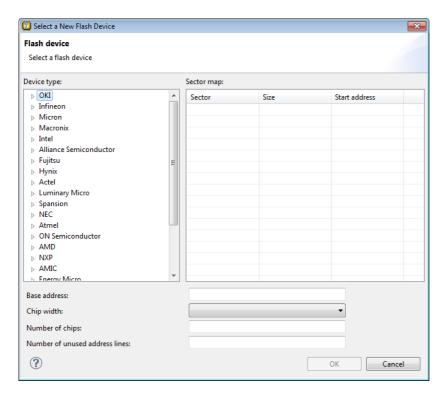
In the Device type box, expand the name of the manufacturer of the device and select a device.
