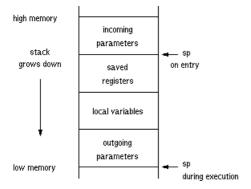
All ARM architectures, except for M-profile architectures, have separate stack pointers for each processor mode. M-profile architectures have one stack pointer. These stack pointers should be initialized at run-time. This is taken care of by the startup code in the run-time library, by means of linker-generated symbols defined in the LSL file. See Section 8.1, *Startup Code*, for a list of these symbols.
