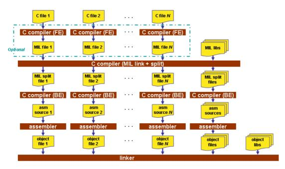
To read more about how MIL linking influences the build process of your application, see Section 12.1, *MIL Linking*.
