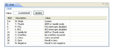
In this view you can set the individual values in the register, either by selecting a value from a drop-down box or by simply entering a value depending on the chosen field. To update the register with the new values, click the **Update** button.
