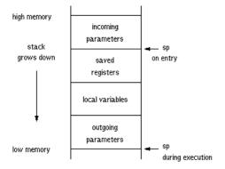
All ARM architectures, except for M-profile architectures, have separate stack pointers for each processor mode. M-profile architectures have one stack pointer. These stack pointers should be initialized at run-time. This is taken care of by the startup code in the run-time library, by means of linker-generated symbols defined in the LSL file. See Section 9.1, Startup Code, for a list of these symbols.
