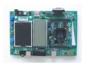
Note that prototype versions of the STM32L152D-EVAL board have some limitations. STMicroelectronic recommends to use SWD instead of JTAG to load and debug the code. For more details see section 1.1 *Prototype limitations* in the *STM32L152D-EVAL evaluation board User Manual.*
