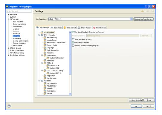
On the **Tool Settings** tab, the options are grouped in Global Options, C/C++ Compiler, Assembler and Linker or Archiver if you are building a library. Note that the options you enter in the Assembler page are not only used for hand-coded assembly files, but also for the assembly files generated by the compiler.
