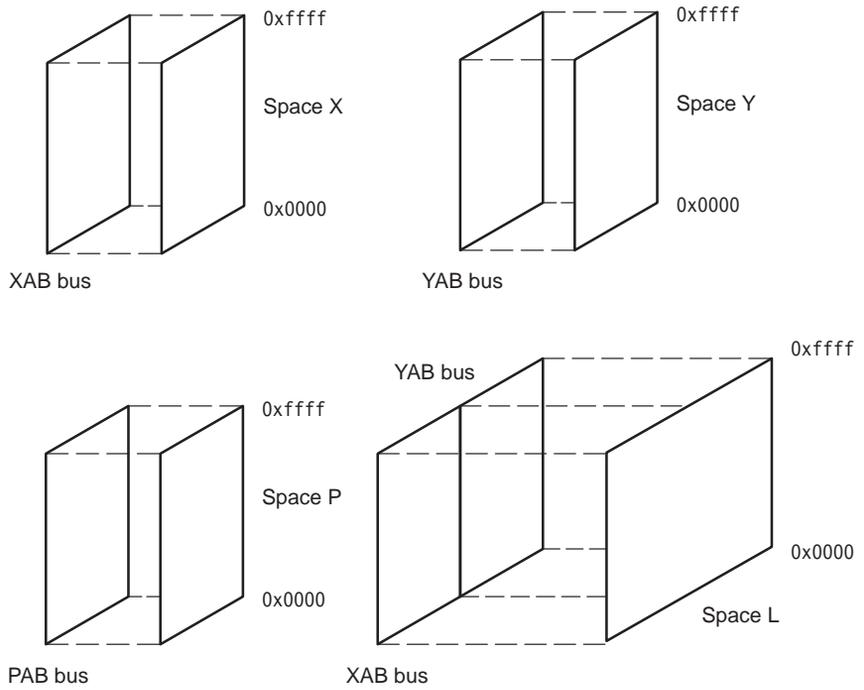
Figure 11-2: DSP5600x physical address space mapping
