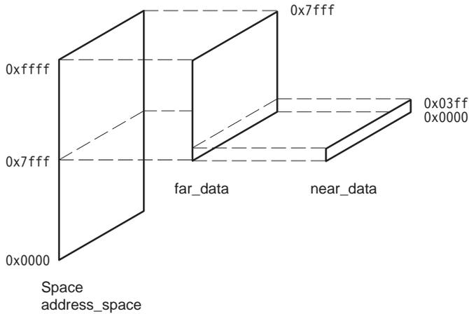
Figure G-3: Addressing mode mapping
