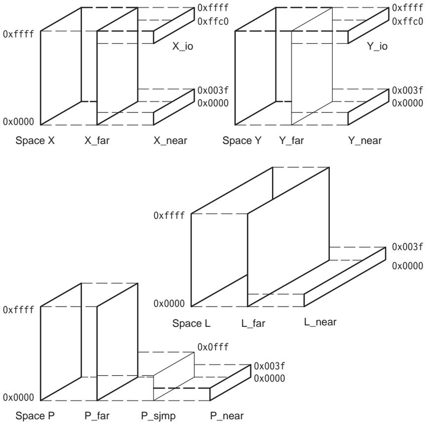
Figure 11-3: DSP5600x virtual address space mapping
