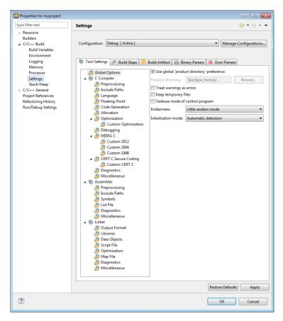
On the **Tool Settings** tab, the options are grouped in Global Options, C Compiler, Assembler and Linker or Archiver if you are building a library. Note that the options you enter in the Assembler page are not only used for hand-coded assembly files, but also for the assembly files generated by the compiler. In the **Configuration** field, you can choose a configuration for which you want to make changes. Note that this does not make the configuration active.
