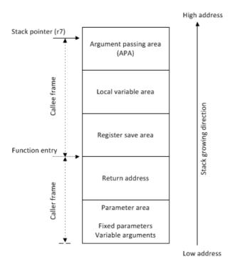
The return address area is used to store the return address of a function call. The register save area is used to store the callee-saves registers when necessary. The local variables area is used to store local variables, function return values and spilled registers. The argument passing area is only used to pass stack parameters to the called functions. After control has been passed to the called function, this area is called the parameter area.
