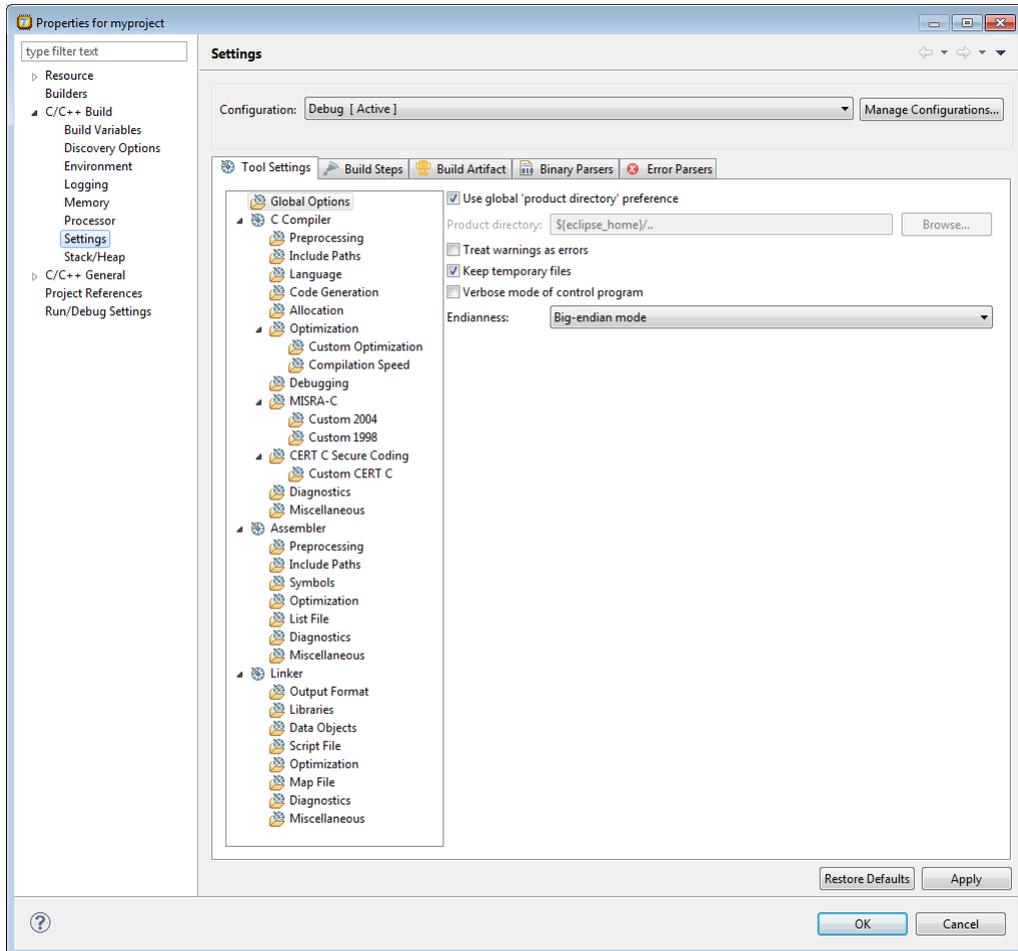
On the **Tool Settings** tab, the options are grouped in Global Options, C Compiler, Assembler and Linker or Archiver if you are building a library. Note that the options you enter in the Assembler page are not only used for hand-coded assembly files, but also for the assembly files generated by the compiler. In the **Configuration** field, you can choose a configuration for which you want to make changes. Note that this does not make the configuration active.
