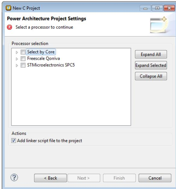
4. Select the target processor for which you want to build the application. You can also make a selection by core. For example, e200z0. Afterwards you can always change the processor in the **Project » Properties for** dialog.
