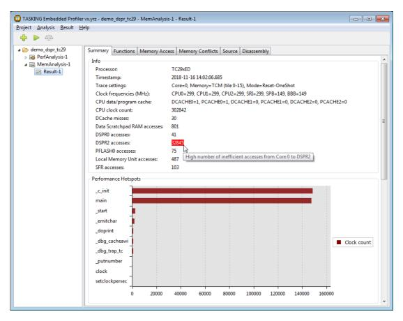
After applying the suggested mitigation, you can use the TASKING Embedded Profiler to confirm that the problem has indeed been fixed. With the default settings of the tool this all happens non-intrusively with real data collected from the application running on the real device. Using such a performance tuning tool, non-expert users can often highly speed up untuned applications.
