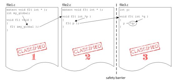
The address of variable  $my_global$  is passed to function f2(). Within function f2(), the address of  $my_global$  is stored in p and passed to function f3(). Within function f3() the address of  $my_global$  is stored in p and dereferenced followed by a read action.
