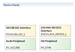
Each colored stack item represents a software module. In this example the ASCLIN stack consists of two modules, for each abstraction level one. In general, your application interfaces only to the highest level modules.
