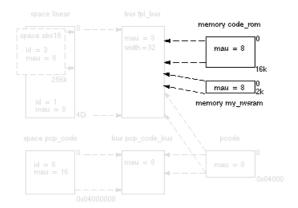
Suppose your embedded system has 16 kB of external ROM, named code\_rom and 2 kB of external NVRAM, named my\_nvsram. Both memories are connected to the bus fpi\_bus. In LSL this looks like:
