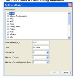
4. In the **Device type** box, expand the name of the manufacturer of the device and select a device.
