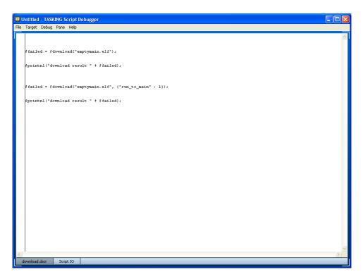
Unless this has already happened, a connection with the target will be established first. Then, provided the script contains no syntax errors, the script itself will run. Output of the script is printed in a separate pane (Script IO in the example above).
