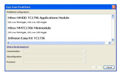
The information in this dialog is based on Debug Target Configuration (DTC) files. DTC files define all possible configurations for a debug target. The files are located in the etc directory of the installed product and use .dtc as filename suffix. For more information on DTC files, see the *TASKING VX-toolset for TriCore User Guide*.
