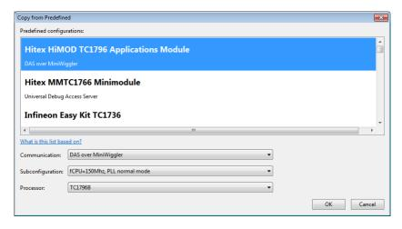
The information in this dialog is based on Debug Target Configuration (DTC) files. DTC files define all possible configurations for a debug target. The files are located in the etc directory of the installed product and use .dtc as filename suffix. For more information on DTC files, see the *TASKING VX-toolset for TriCore User Guide*.
