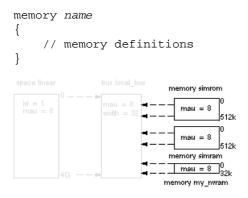
Suppose your embedded system has 512kB of external ROM, named simrom, 512kB of external RAM, named simram and 32kB of external NVRAM, named my\_nvram (see figure above.) All memories are connected to the bus local\_bus. In LSL this looks like follows:
