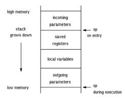
All ARM architectures, except for M-profile architectures, have separate stack pointers for each processor mode. M-profile architectures have one stack pointer. These stack pointers should be initialized at run-time. This is taken care of by the startup code in the run-time library, by means of linker-generated symbols defined in the LSL file. See Section 9.1, *Startup Code*, for a list of these symbols.
