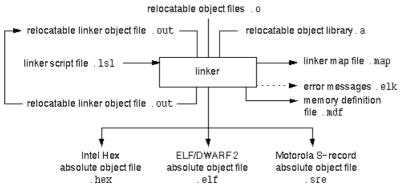
This chapter first describes the linking process. Then it describes how to call the linker and how to use its options. An extensive list of all options and their descriptions is included in Section 8.3, *Linker Options*.
