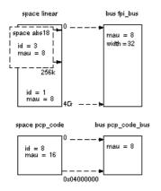
The figure shows three address spaces called linear, abs18 and pcp\_code. The address space abs18 is a subset of the address space linear. All address spaces have attributes like a number that identifies the logical space (id), a MAU and an alignment. In LSL notation the definition of these address spaces looks as follows:
