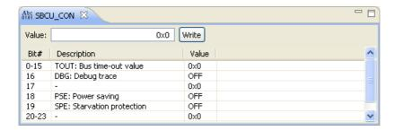
In this view you can set the individual values in the register, either by selecting a value from a drop-down box or by simply entering a value depending on the chosen field. To update the register with the new values, click the **Write** button.
