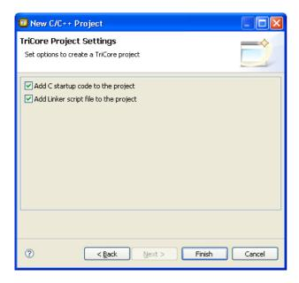
This adds the files <code>cstart.c</code> and <code>cstart.h</code> to your project. These files are copies of <code>lib/src/cstart.c</code> en <code>include/cstart.h</code>. If you do not add the startup code here, you can always add it later with <code>File » New » Other... » TASKING C/C++ » cstart.c/cstart.h Files.</code>
