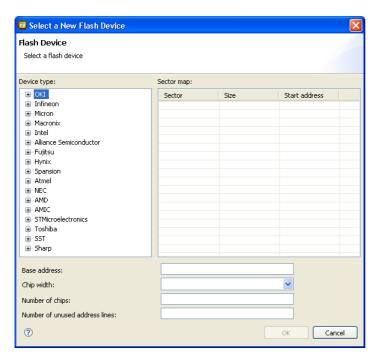
4. In the **Device type** box, expand the name of the manufacturer of the device and select a device.
