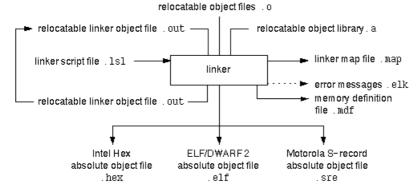
This chapter first describes the linking process. Then it describes how to call the linker and how to use its options. An extensive list of all options and their descriptions is included in Section 11.4, *Linker Options*.
