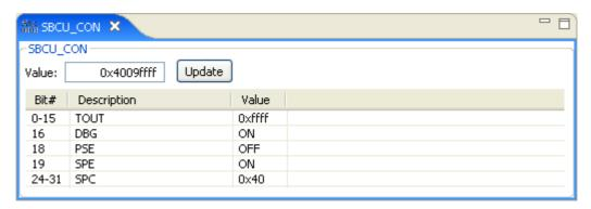
In this view you can set the individual values in the register, either by selecting a value from a drop-down box or by simply entering a value depending on the chosen field. To update the register with the new values, click the **Update** button.
