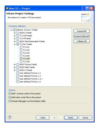
This adds the files <code>cstart.c</code> and <code>cstart.h</code> to your project. These files are copies of <code>lib/src/cstart.c</code> and <code>include/cstart.h</code>. If you do not add the startup code here, you can always add it later with <code>File » New » cstart.c/cstart.h Files</code>.
