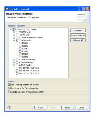
This adds the files <code>cstart.c</code> and <code>cstart.h</code> to your project. These files are copies of <code>lib/src/cstart.c</code> and <code>include/cstart.h</code>. If you do not add the startup code here, you can always add it later with <code>File » New » cstart.c/cstart.h Files</code>.
