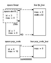
The figure shows three address spaces called linear, abs18 and pcp\_code. The address space abs18 is a subset of the address space linear. All address spaces have attributes like a number that identifies the logical space (id), a MAU and an alignment. In LSL notation the definition of these address spaces looks as follows:
