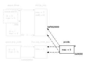
According to the drawing, the TriCore contains internal memory called pcode with a size 0x04000 (16 kB). This is physical memory which is mapped to the internal bus  $pcp\_code\_bus$  and to the fpi\\_bus, so both the tc unit and the PCP can access the memory:
