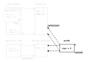
According to the drawing, the TriCore contains internal memory called pcode with a size 0x04000 (16 kB). This is physical memory which is mapped to the internal bus pcp\_code\_bus and to the fpi\_bus, so both the tc unit and the PCP can access the memory:
