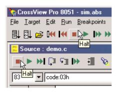
The simulator runs one line, stops, updates the windows and continues again. This is a very simple way to verify whether the example runs correctly. As it can take a very long time to run all the code, however, it is better to stop the simulator at this point by clicking on either of the two **HALT** buttons and to take a closer look at some of the options of the source window.
