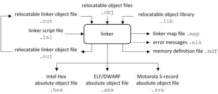
The linker takes the following files for input and output:
