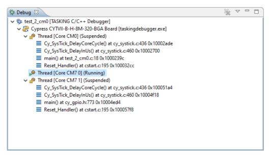
For each of the cores CM0, CM7 0 and CM7 1 a separate thread is started. The example shows the situation where Thread [Core CM0] is suspended, Thread [Core CM7 0] is running and Thread [Core CM7 1] is suspended.
