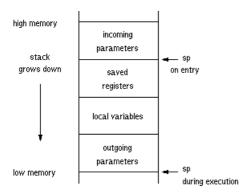
All ARM M-profile architectures have one stack pointer. This stack pointer should be initialized at run-time. This is taken care of by the startup code in the run-time library, by means of the linker-generated symbol \_lc\_ub\_stack defined in the LSL file. See Section 8.1, *Startup Code*.
