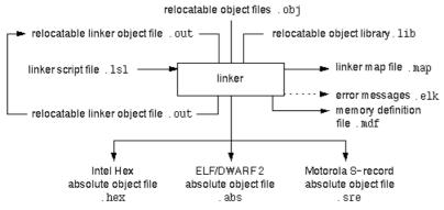
This chapter first describes the linking process. Then it describes how to call the linker and how to use its options. An extensive list of all options and their descriptions is included in Section 13.5, *Linker Options*.
