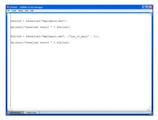
Unless this has already happened, a connection with the target will be established first. Then, provided the script contains no syntax errors, the script itself will run. Output of the script is printed in a separate pane (Script IO dac in the example above).
