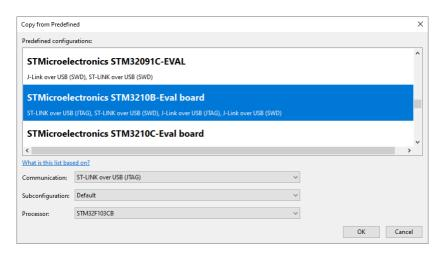
The information in this dialog is based on Debug Target Configuration (DTC) files. DTC files define all possible configurations for a debug target. The files are located in the etc directory of the installation directory or a vendor specific Eclipse plugin
