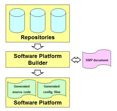
A Software Platform repository may contain any kind of software, but typical modules include interrupt services, timers, peripherals (hardware wrappers), drivers, kernel services (such as POSIX multithreading), device I/O, file system (FatFs), networking (TCP/IP), graphical user interface, etc.
