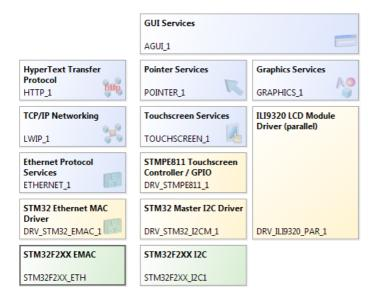
Each colored stack item represents a software module. In this example the HTTP stack consists of five modules, for each abstraction level one. The GUI Services requires Graphics Services and Pointer Services. In general, your application interfaces only to the highest level modules.
