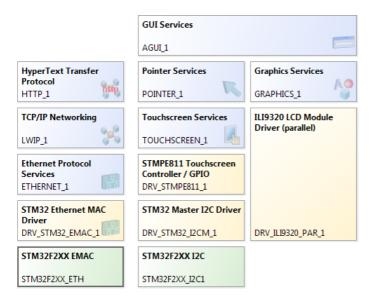
Note that some drivers (ILI9320 LCD Module Driver in this example) do not require a peripheral, because the device is accessed through the memory controller.
