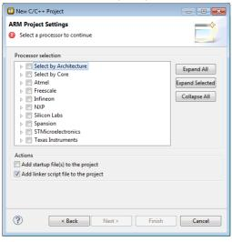
Select the target processor core or architecture for which you want to build the application. In this
