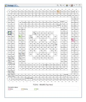
A square around a pin marks the selected pin. In the package above P00.0 is selected. A green check mark indicates that the pin has a valid connection; P00.0 and P01.6 in the package above. A red cross
