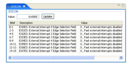
In this view you can set the individual values in the register, either by selecting a value from a drop-down box or by simply entering a value depending on the chosen field. To update the register with the new values, click the **Update** button.
