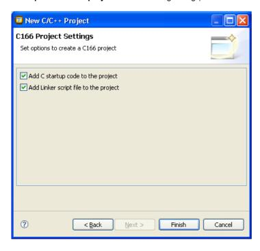
This adds the files <code>cstart.c</code> and <code>cstart.h</code> to your project. These files are copies of <code>lib/src/cstart.c</code> en <code>include/cstart.h</code>. If you do not add the startup code here, you can always add it later with <code>File > New > Other... > TASKING C/C++ > cstart.c/cstart.h</code> Files.
