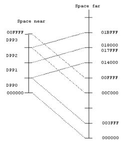
The figure shows two address spaces called near and far. All address spaces have attributes like a number that identifies the logical space (id), a MAU and an alignment. In LSL notation the definition of these address spaces looks as follows:
