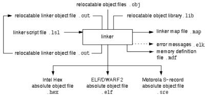
This chapter first describes the linking process. Then it describes how to call the linker and how to use its options. An extensive list of all options and their descriptions is included in Section 12.5, *Linker Options*.
