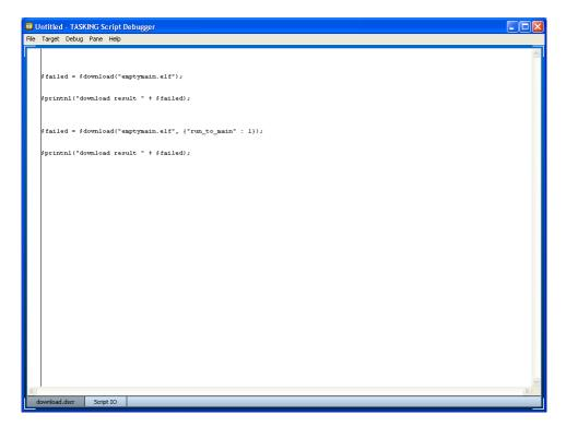
Unless this has already happened, a connection with the target will be established first. Then, provided the script contains no syntax errors, the script itself will run. Output of the script is printed in a separate pane (Script IO in the example above).
