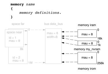
Figure 8-3: Adding external memory to the M16C architecture
