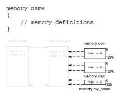
Suppose your embedded system has 128kB of external ROM, named xrom, 128kB of external RAM, named xram and 32kB of external NVRAM, named my\_nvram (see figure above.) All memories are connected to the bus local\_bus. In LSL this looks like follows:
