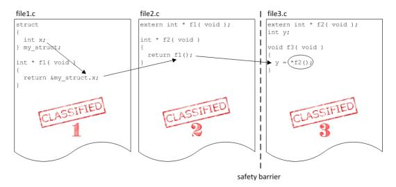
The address of a structure member is returned by function f1() in module 1. The return value of f1() is returned by function f2() in module 2. And function f3() in module 3 reads the content of the address returned by function f2().
