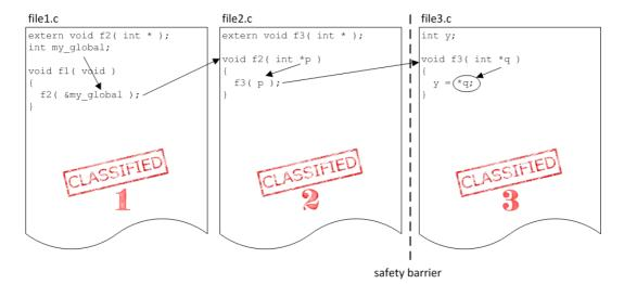
The address of variable  $my_global$  is passed to function f2(). Within function f2(), the address of  $my_global$  is stored in p and passed to function f3(). Within function f3() the address of  $my_global$  is stored in q and dereferenced followed by a read action.
