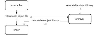
The linker optionally includes object modules from a library if that module resolves an external symbol definition in one of the modules that are read before.
