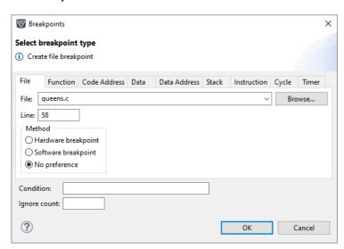
If a debug session is active, the **File** drop-down box is filled with all source files as present in the debug information in the ELF file. This can include files not present in the Eclipse project (for example from libraries). If a file could be matched to a file in the active Eclipse project it will show as an Eclipse project relative filename.
