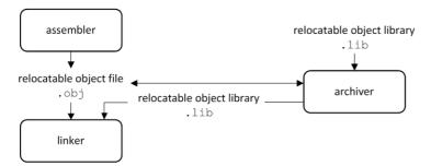
The linker optionally includes object modules from a library if that module resolves an external symbol definition in one of the modules that are read before.
