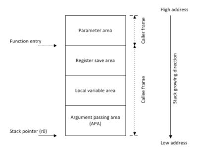
The register save area is used to store the callee-saves registers when necessary. The local variables area is used to store local variables, function return values and spilled registers. The argument passing
