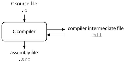
This chapter first describes the compilation process which consists of a *frontend* and a *backend* part. Next it is described how to call the C compiler and how to use its options. An extensive list of all options and their descriptions is included in [Section 8.1, C Compiler Options](#). Finally, a few important basic tasks are described, such as including the C startup code and performing various optimizations.
