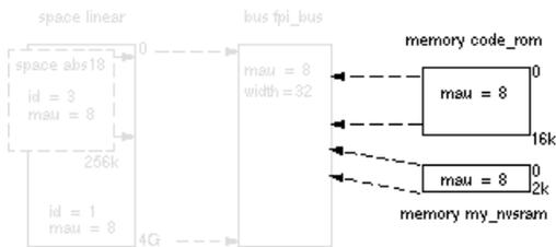
Suppose your embedded system has 16 kB of external ROM, named `code_rom` and 2 kB of external NVRAM, named `my_nvram`. Both memories are connected to the bus `fpi_bus`. In LSL this looks like:
