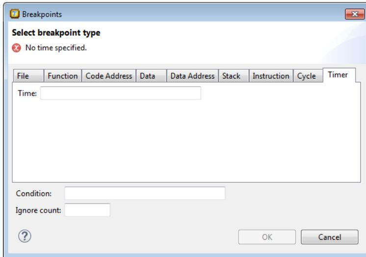
The target halts when the given amount of **Time** elapsed. The value entered is interpreted by the debug instrument.
