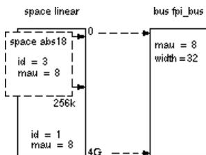
The figure shows two address spaces called `linear` and `abs18`. The address space `abs18` is a subset of the address space `linear`. All address spaces have attributes like a number that identifies the logical
