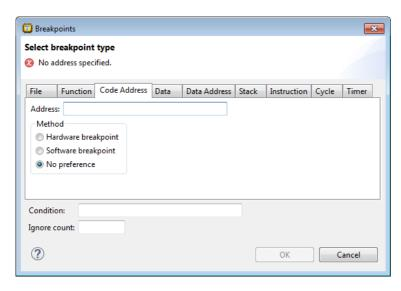
The target halts when it reaches the specified instruction address.
