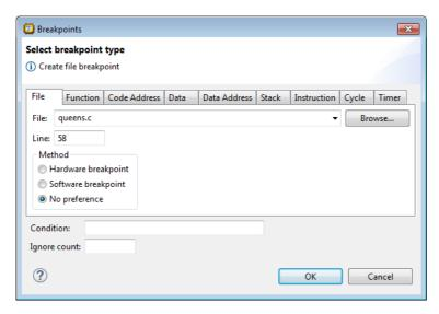
If a debug session is active, the **File** drop-down box is filled with all source files as present in the debug information in the ELF file. This can include files not present in the Eclipse project (for example from libraries). If a file could be matched to a file in the active Eclipse project it will show as an Eclipse project relative filename.
