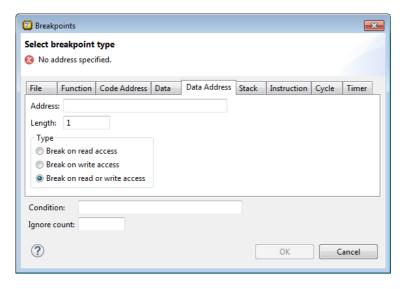
The target halts when the given memory range (specified in terms of an absolute **Address** and a **Length** in MAUs) is read or written to, as specified.
