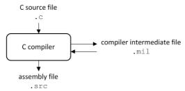
This chapter first describes the compilation process which consists of a *frontend* and a *backend* part. Next it is described how to call the C compiler and how to use its options. An extensive list of all options and their descriptions is included in Section 8.2, *C Compiler Options*. Finally, a few important basic tasks are described, such as including the C startup code and performing various optimizations.
