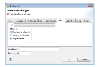
The target halts when it reaches the specified stack level.
