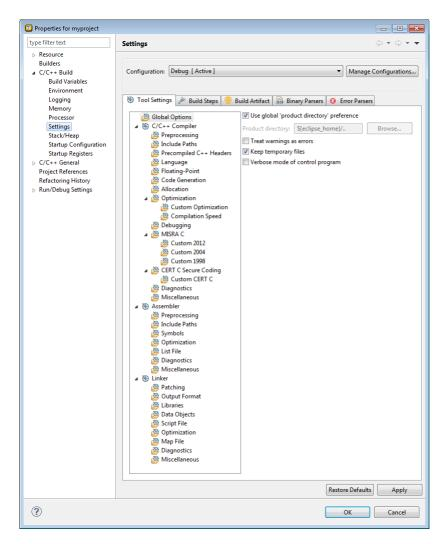
On the **Tool Settings** tab, the options are grouped in Global Options, C/C++ Compiler, Assembler and Linker or Archiver if you are building a library. Note that the options you enter in the Assembler page are not only used for hand-coded assembly files, but also for the assembly files generated by the compiler. In the **Configuration** field, you can choose a configuration for which you want to make changes. Note that this does not make the configuration active.
