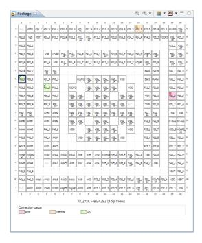
A square around a pin marks the selected pin. In the package above P00\_0 is selected. A green check mark indicates that the pin has a valid connection; P00\_0 and P01\_6 in the package above. A red cross indicates an error; P21\_3 in the package above. A triangle with exclamation mark indicates a warning; P14\_4 in the package above. When you click on a pin, the pin appears in the editor. If the pin contains an error, you can see what is wrong in the Pin Conflicts view.
