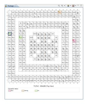
A square around a pin marks the selected pin. In the package above P00\_0 is selected. A green check mark indicates that the pin has a valid connection; P00\_0 and P01\_6 in the package above. A red cross
