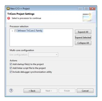
This adds the files <code>cstart.c</code> and <code>cstart.h</code> to your project. These files are copies of <code>lib/src/cstart.c</code> and <code>include/cstart.h</code>. If you do not add the startup code here, you can always add it later with <code>File » New » Startup Files</code>.
