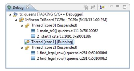
For each of the three TriCore cores of the TC29x a separate thread is started. The example shows the situation where Thread [core 0] is suspended, Thread [core 1] is running and Thread [core 2] is suspended.
