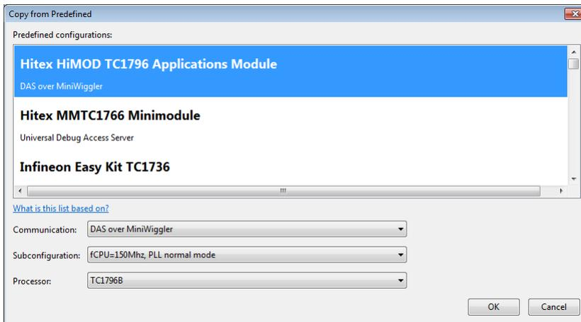
The information in this dialog is based on Debug Target Configuration (DTC) files. DTC files define all possible configurations for a debug target. The files are located in the `etc` directory of the installed product and use `.dtc` as filename suffix. For more information on DTC files, see the *TASKING VX-toolset for TriCore User Guide*.
