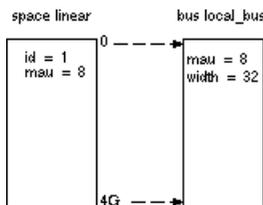
The figure shows one address space called `linear`. The address space has attributes like a number that identifies the logical space (id), a MAU and an alignment. In LSL notation the definition of this address space looks as follows:
