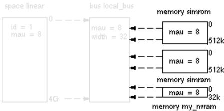
Suppose your embedded system has 512kB of external ROM, named `simrom`, 512kB of external RAM, named `simram` and 32kB of external NVRAM, named `my_nvram` (see figure above.) All memories are connected to the bus `local_bus`. In LSL this looks like follows:
