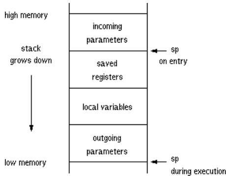
All ARM architectures, except for M-profile architectures, have separate stack pointers for each processor mode. M-profile architectures have one stack pointer. These stack pointers should be initialized at run-time. This is taken care of by the startup code in the run-time library, by means of linker-generated symbols defined in the LSL file. See [Section 9.1, Startup Code](#), for a list of these symbols.
